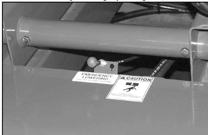
Figure 5: Emergency Lowering Knob, LX31 and LX41
